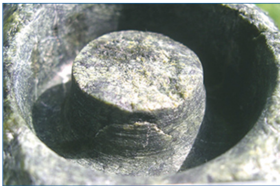
Figure 13: Experimental bore core which appears in the centre of the tube during the drilling operation
