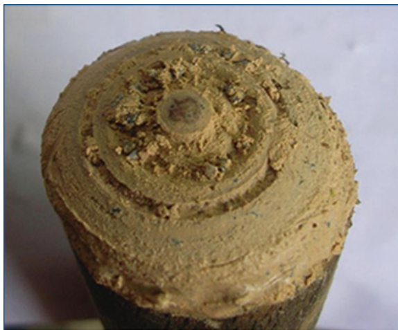
Figure 15: End of a solid wooden drill bit
