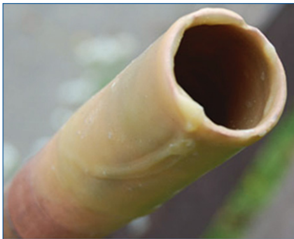
Figure 14: Experimental copper tube coated with wax
